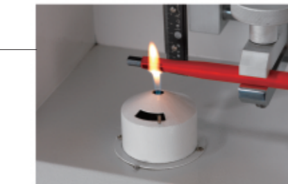
The low flammability properties of insulated T-handle material makes the height of flame not exceed 120mm within 20 second.
